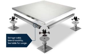
The pedestals are of a Zinc plated steel construction, ensuring electrical continuity, pre-assembled to help minimize installation time. The pedestals have a locking nut to ensure that once adjusted and locked there is no movement in the pedestal head.
